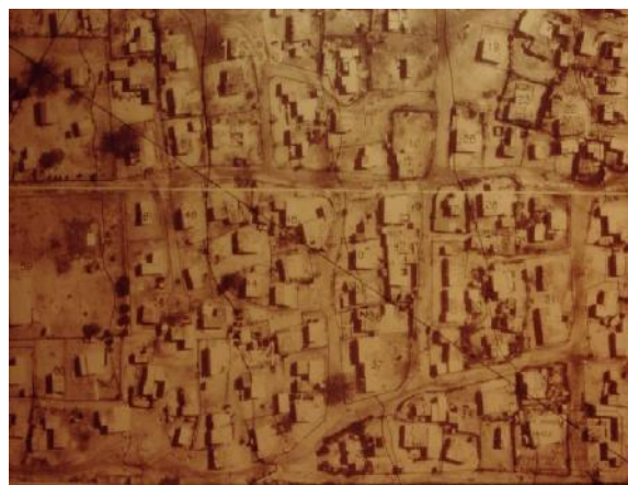
Figure 3: Shows a preliminary attempt at identifying points of intersection of straights which define the boundaries between properties marked on the orthophoto using a Cad system.
