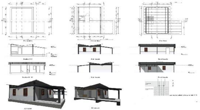
Figure 10: Butterfly House as a core house equipped with simple cladding (drawing by the authors)
